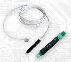
The sensor is designed to measure temperature and humidity with 1-wire bus communication. Thanks to its narrow design, it is suitable for use in narrow spaces such as risers, shafts or RACK cabinets and therefore it can be used, for example, for measurements in data centers or server rooms. The 4-core PVC "telephone" cable is terminated with an RJ11 connector as standard, but the sensor can also be supplied without a cable terminated with a connector.
