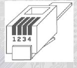
Terminal 1....... Not used Terminal 2....... 1-wire (data) Terminal 3...... GND Terminal 4....... + 5V (Ucc)
