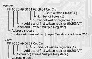
(module with embedded jumper "service" - address 255) Writing data 0x0904 to the register 0x200 A\*\* is set address 9
