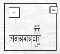
K1....connection sensor T+RH K2...connector USb mini B
