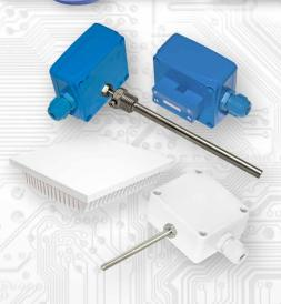
Temperature sensors KTY81 are available in following versions - interior, outdoor, duct, screw-in, surface contact, cable sensors. The transducer's head is made of the plastic material, cover is provided with quick-locking screws, all metallic parts are made of class DIN 1.4301 stainless steel. The operation conditions are met by conventional, chemically non aggressive environment, in which neither attendance nor maintenance is required by the transducers.
