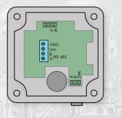
jumper A...definition of still stand (conductor A) jumper B...definition of still stand (conductor B) jumper ZAK ...terminal resistor 120R jumper J6 ... device configuration jumper J7 ... definition of diagnostic network mode Term. A, B... RS485 Term. Ucc... power supply Term. GND... common pole
