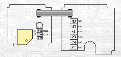
J7... ACDL (Automatic Calibration in Dimming Light mode)
