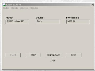
With clicking on the "READ" button opens the window with the current input values.
