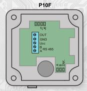
jumper A...definition of still stand (conductor A) jumper B...definition of still stand (conductor B)
