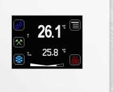
The controller RK-HTM-D is an interior device intended for sensing, and possible correction, of environment temperature and relative humidity of air without aggressive admixtures.
