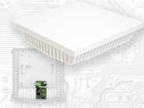
The sensors are designed to measure relative air humidity and possibly air temperature without aggressive additives in interiors with increased aesthetic demands. They are adapted for direct mounting on an interior wall or on a standard installation box with a spacing of 60mm.
