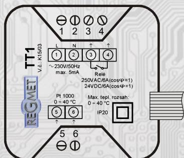
Terminals 1 and 2..... power supply 230 V / 50 Hz
