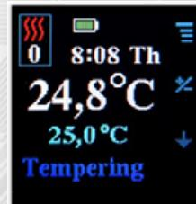
In the initial condition, the thermostat is set to room heating mode with PI control, with a control period of 10 min., and tempering mode to 20°C. This means that only the interior temperature is measured and controlled to 20°C without any time profiles.
