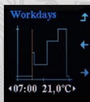
By pressing **←** and **→**, you can scroll between individual stamps; the time and temperature of the selected stamp is shown on the bottom line. By pressing **↑**, you can return back. Using the same procedure, you can set the profiles for weekend or holidays. By selecting **↑ Activate and pressing ↻**, you activate given profile. By selecting **▶ Back and pressing ↻**, you return back by one menu level (this applies for the entire menu: by selecting **▶ Back**, you can return one step back).
