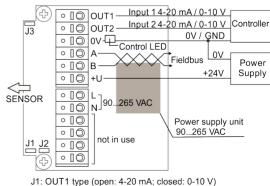
J1: OUT1 type (open: 4-20 mA; closed: 0-10 V) J2: OUT2 type (open: 4-20 mA; closed: 0-10 V)
